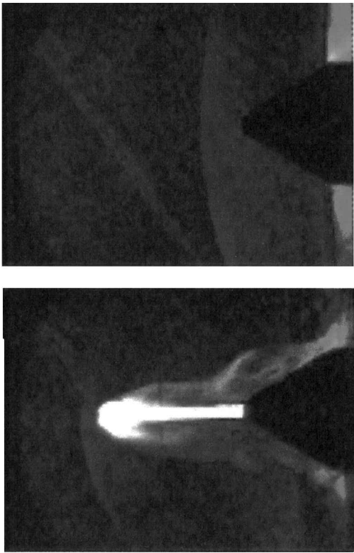
Fig. 3 Shadowgraphs at M_\infty = 1.18 prior to (top) and at the instant of plasma discharge.
